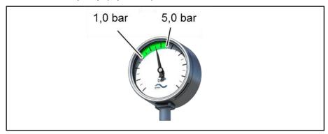
Figure 15: Inlet pressure gauge
