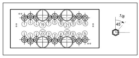
Figure 18: Tightening sequence for screw connections
