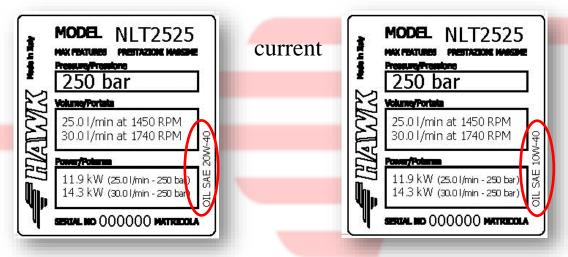
SAE 10W-40 oil has been unified in the whole Hawk production, to provide better performance at low temperature regimes. Better lubrication and less splash lubricated during start-up.
