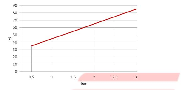
Note how a supply pressure of 3 bar extends the life of the pump (seals and valves), even with low liquid temperatures (for example 45°C).
