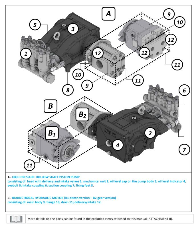
The pumping action is created by a series of plungers, connected to the drive shaft by connecting rods. During motion, the plungers slide on their axis inside the manifold housing where the suction and delivery lines are fitted with valves that allow the liquid to flow in a single direction.
