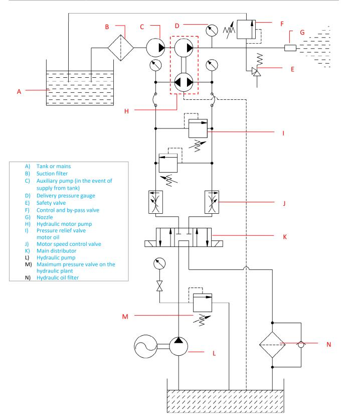
All the hydraulic motors used with Hawk motor pumps are bidirectional.
